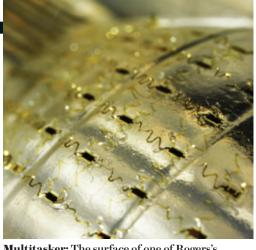
Multitasker: The surface of one of Rogers's balloon catheters is covered with electrodes.
